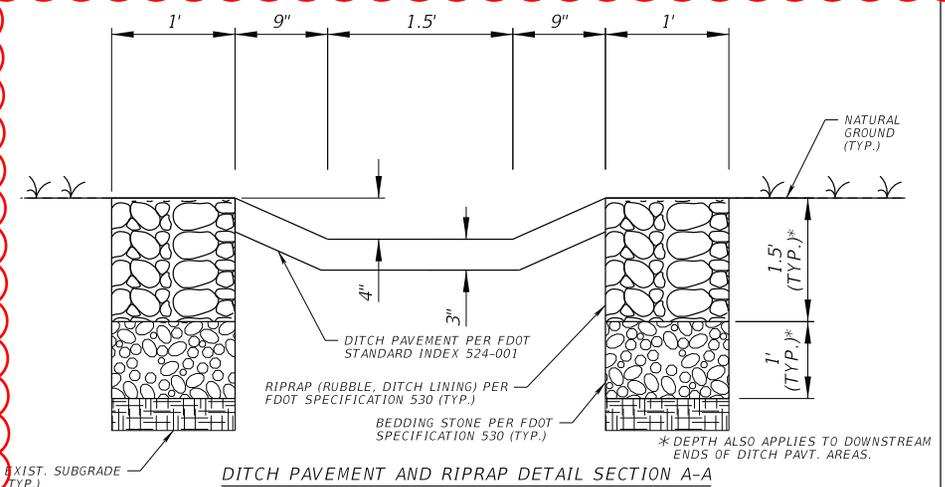
DITCH PAVEMENT AND RIPRAP DETAIL SECTION A-A
