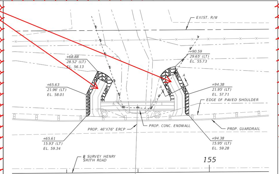
CROSS DRAIN AT STA. 144+77.88 DITCH PAVEMENT AND RIPRAP DETAIL (SCALE: 1" = 10')
